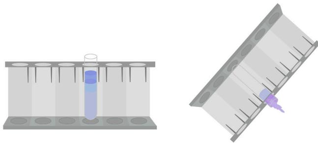
Figure 4: Hand-decanting supernatant using a Magnetic Rack.
